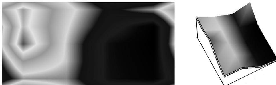
Fig. 5. Raman mapping of RBM band. Comparison between a top view (left panel) and a 3D view (right panel). The grayscale indicates the intensities of the band. Laser excitation 785 nm
